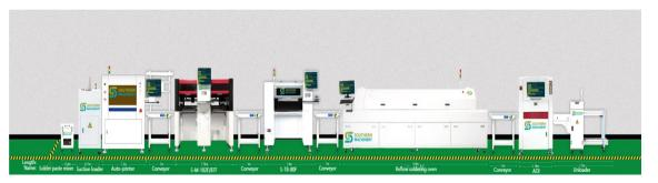
8 Spindle + 4 Spindle Production Line 35000CPH
